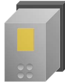
Drive mounted on a “footprint” filter
